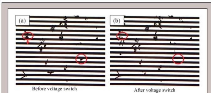
**Figure 16.** Images captured with a digital microscope of CFC powder on the surface of (a) an uncharged tri-polar grid and (b) a charged tri-polar grid. The red circles indicate some particles have been moved.
