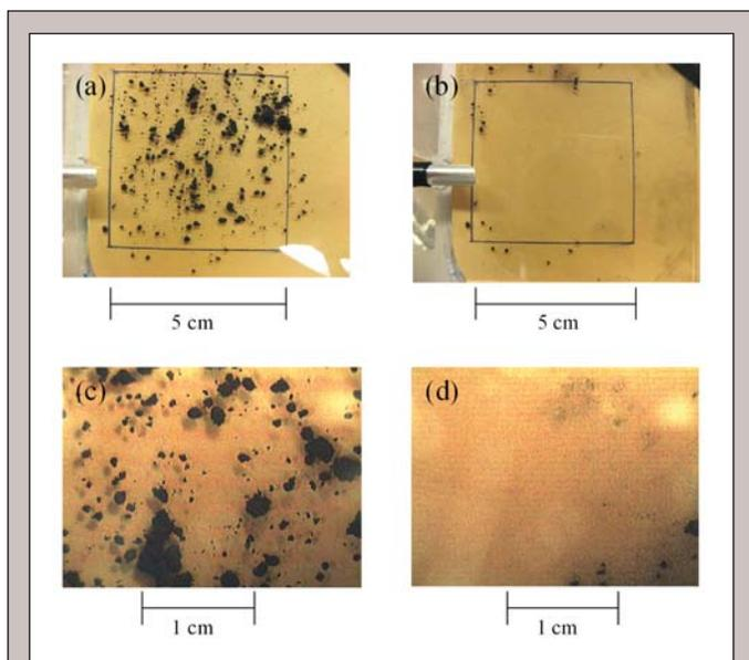
**Figure 11.** Pictures of carbon particles at atmospheric pressure taken (a) with digital camera before puff, (b) with digital camera after puff, (c) with digital microscope before puff and (d) with digital microscope after puff.
