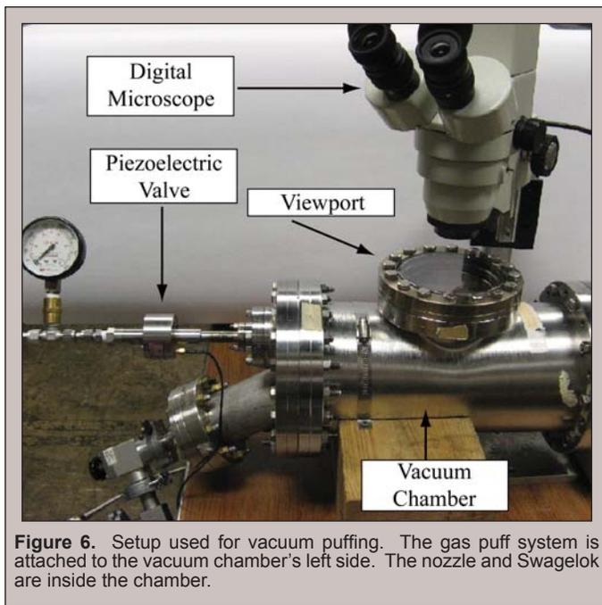
**Figure 6.** Setup used for vacuum puffing. The gas puff system is attached to the vacuum chamber's left side. The nozzle and Swagelok are inside the chamber.
