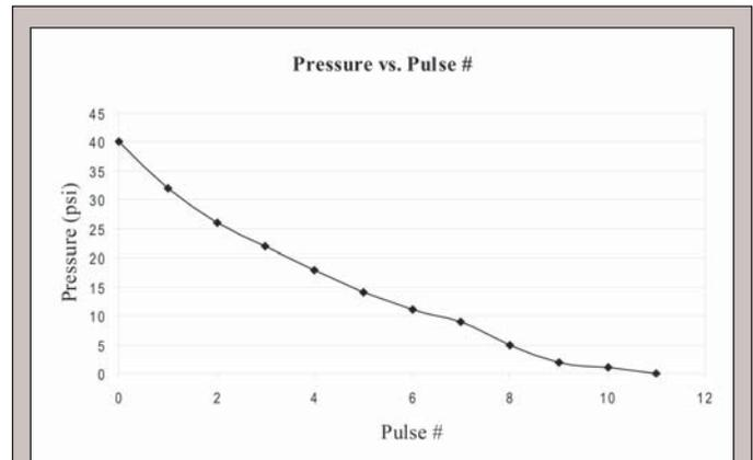
**Figure 8.** Backing pressure vs. number of pulses supplied. As expected, the pressure decreased as more pulses were provided. The pulse amplitude used for this test was 170 V.
