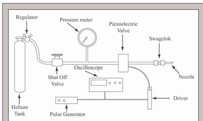
**Figure 2.** Schematic of the gas puff system, not to scale. Helium gas was blown through the system and was expelled at a  $45^\circ$  angle through the nozzle.
