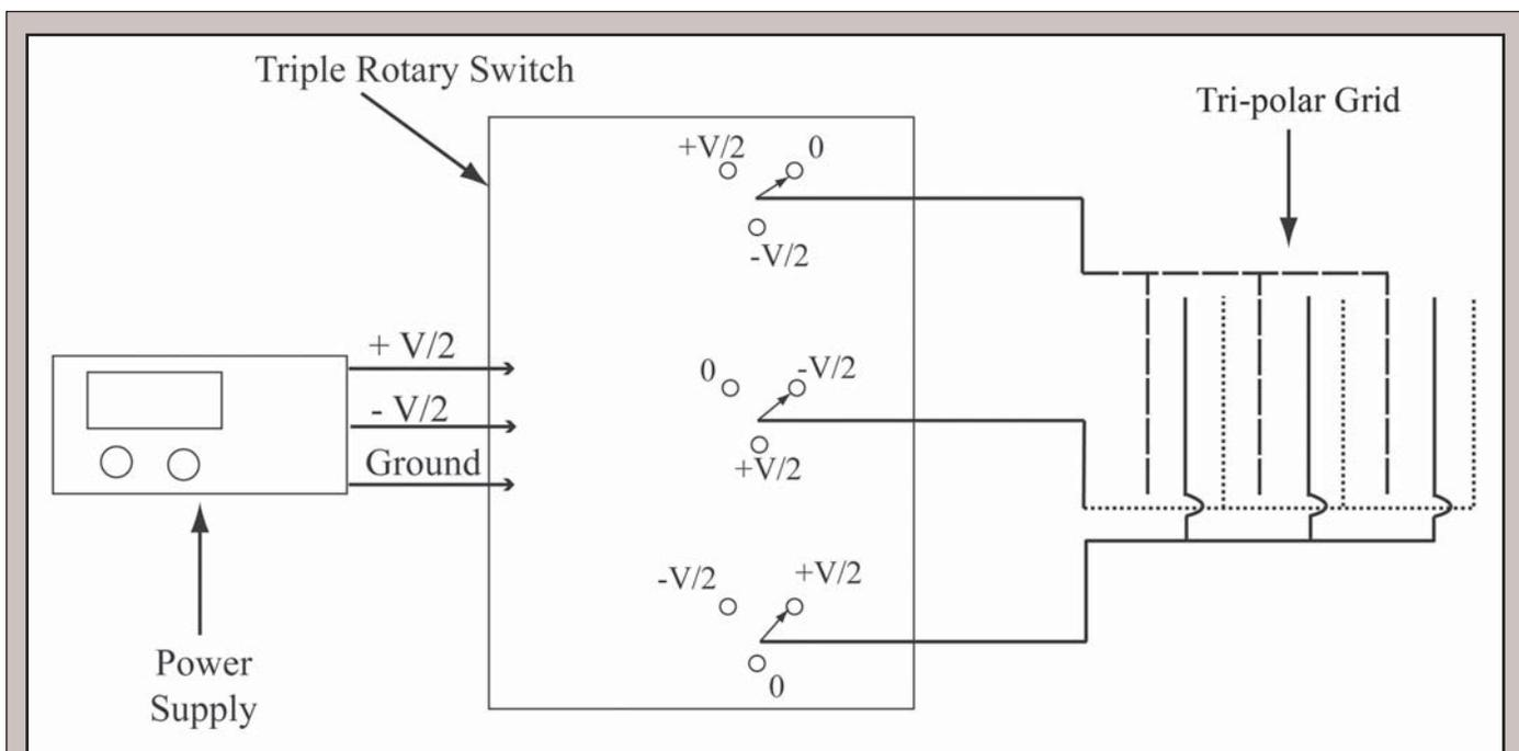
**Figure 3.** Schematic of the electrostatic dust transporter system. Dashed lines were used to differentiate between the three electrodes.
