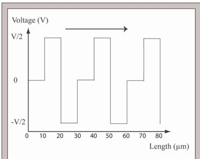
**Figure 4.** Schematic of the traveling electrostatic wave on the tri-polar grid with gold traces. The potential gradient is created by three different voltages on the three electrodes.
