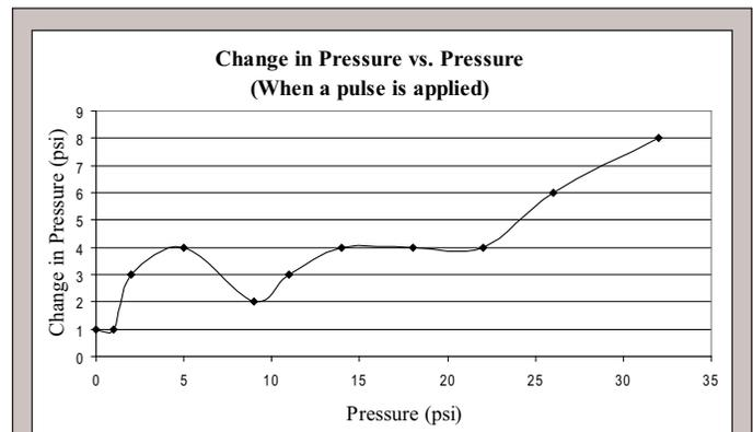
**Figure 9.** Change in pressure vs. backing pressure. For each pulse given, there is a big pressure drop when the backing pressure is high. Similarly, the pressure drop is small when the backing pressure is low.
