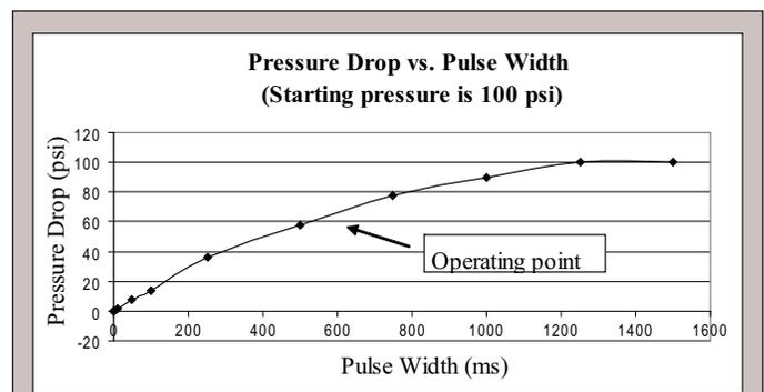
**Figure 10.** Pressure drop vs. pulse width. A large pulse width gives bigger backing pressure drops. All pressure drops were in reference to an initial backing pressure of 100 psi. The pulse width chosen for gas puffing was 500 ms.
