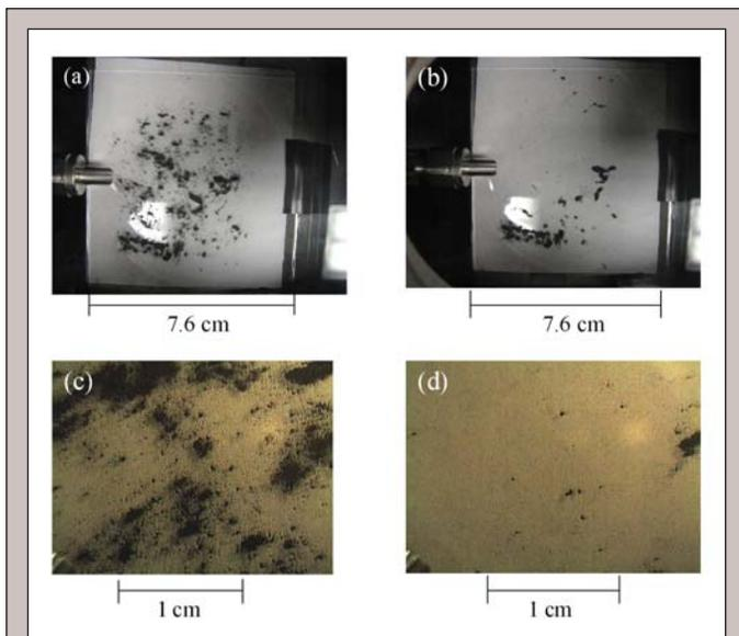
**Figure 15.** Pictures of tungsten particles at base vacuum pressure of 1 mTorr taken (a) with digital camera before puff, (b) with digital camera after puff, (c) with digital microscope before puff and (d) with digital microscope after puff.
