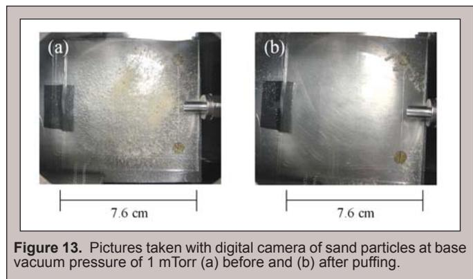
**Figure 13.** Pictures taken with digital camera of sand particles at base vacuum pressure of 1 m Torr (a) before and (b) after puffing.
