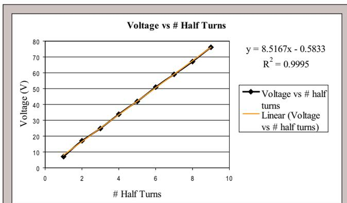
**Figure 7.** Driver output voltage vs. control knob. The oscilloscope had a maximum voltage range of 80 V. Higher voltage pulses produced by the driver were not observed with an oscilloscope, but were predicted with a linear fit shown on the upper right corner of the graph.
