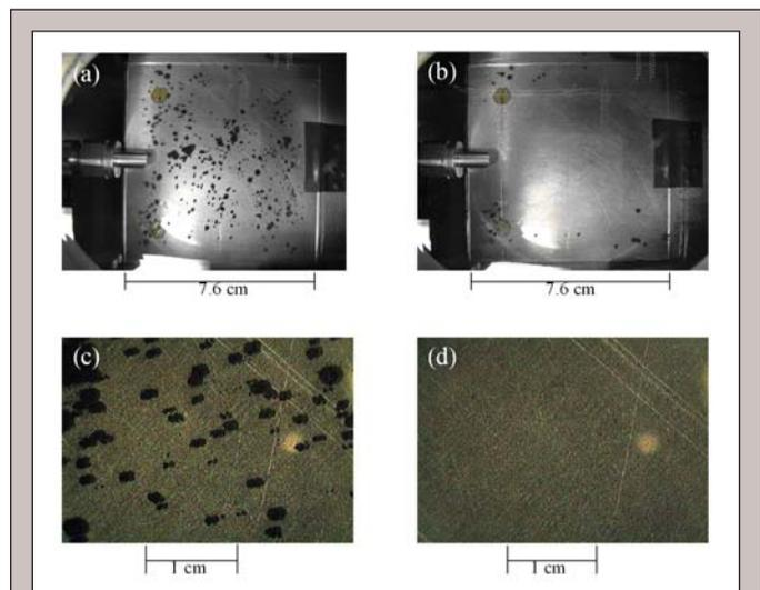
**Figure 14.** Pictures of carbon particles at base vacuum pressure of 1 m Torr taken (a) with digital camera before puff, (b) with digital camera after puff, (c) with digital microscope before puff and (d) with digital microscope after puff.
