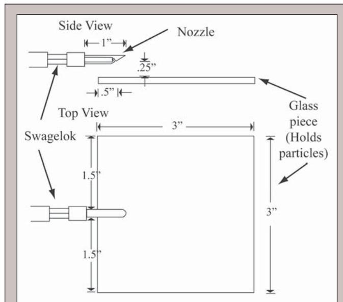
**Figure 5.** Schematic of setup used for tests to obtain the optimum backing pressure, voltage pulse width and nozzle exit channel diameter.
