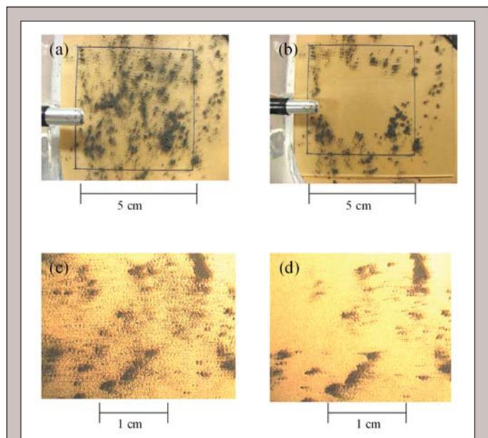
**Figure 12.** Pictures of tungsten particles at atmospheric pressure, taken (a) with digital camera before puff, (b) with digital camera after puff, (c) with digital microscope before puff and (d) with digital microscope after puff.
